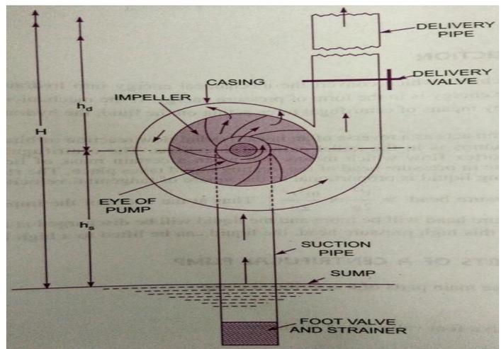
a) **Volute Casing:** It is the casing surrounding the impeller. It is of a spiral type, in which area of flow increases gradually. The increase in area of flow decreases the velocity of flow. The decrease in velocity increases the pressure of the water flowing through the casing. It has been observed that in case of volute casing, the efficiency of the pump increase slightly as a large amount of energy is lost due to the formation of eddies in this type of casing.
