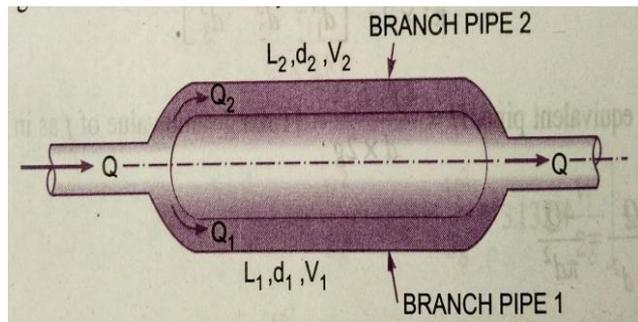
The rate of discharge in the main line is equal to the sum of the discharges in each of the parallel pipes.
