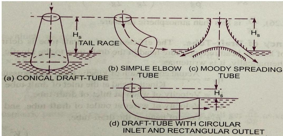
and moody spreading draft tubes are most efficient while simple elbow draft tube and elbow draft tubes with circular inlet and rectangular outlet require less space as compared to other draft tubes.
