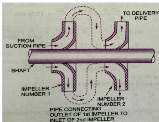
**Multi-Stage Centrifugal Pumps for High Heads:** For developing a high head, a number of impellers are mounted in series on the same shaft.
