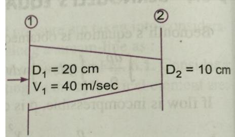
4 Water is flowing through a pipe having diameters 20cms and 10cms at sections 1 and 2 respectively. The rate of flow through pipe is 35 liters/sec. The section 1 is 6m above the datum and section 2 is 4m above the datum. If the pressure at section 1 is 39.24n/cm<sup>2</sup>. Find the intensity of pressure at section 2?
