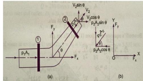
And  $V_2, P_2, A_2$  are corresponding values of Velocity, Pressure, Area at section (2)
