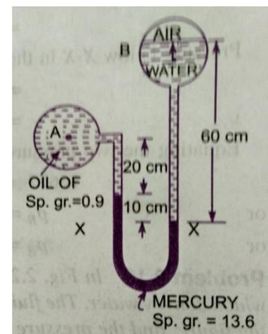
10. A differential manometer is connected at two points A and B. At B air pressure is  $9.81 \text{ N/cm}^2$ . Find absolute pressure at A.
