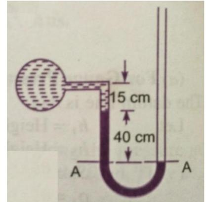
7. What are the gauge pressure and absolute pressure at a point 3m below the surface of a liquid having a density of  $1.53 \times 10^3 \text{ kg/m}^3$ ? If the atmospheric pressure is equivalent to 750mm of mercury. The specific gravity of mercury is 13.6 and density of water  $1000 \text{ kg/m}^3$
