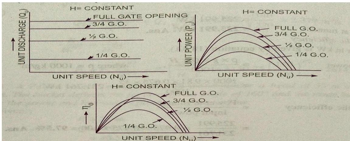
Fig. 18.35 Main characteristic curves for a Pelton wheel.
