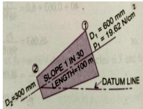
$$\text{Rate of flow } Q = 50 \text{ Lts/sec} = \frac{50}{1000} = 0.05 \text{ m}^3/\text{sec}$$
