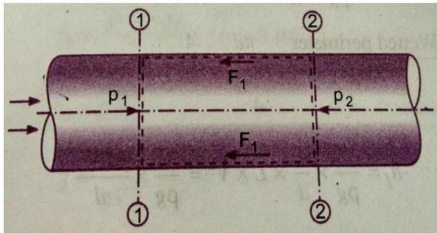
Consider a uniform horizontal pipe having steady flow. Let 1-1, 2-2 are two sections of pipe.
