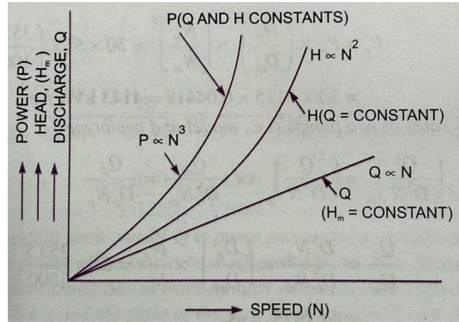
For plotting the curve of  $H_m$  versus speed ( $N$ ) the discharge is kept constant. From the equation it is clear that  $\frac{H_m}{DN}$  is a constant or  $H_m \propto N^2$ . This means that the head developed by a pump is proportional to  $N^2$ . Hence the curve of  $H_m$  v/s  $N$  is a parabolic curve.
