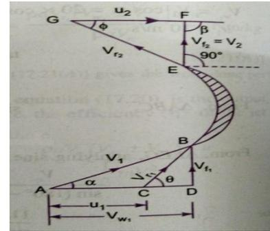
Vane angles at inlet and outlet are  $\theta$  and  $\phi$
