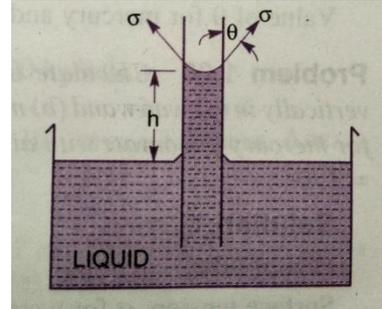
The weight of the liquid of height 'h' in the tube
