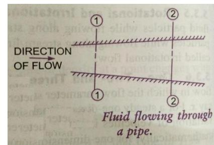
$$\rho_1 A_1 V_1 = \rho_2 A_2 V_2$$
