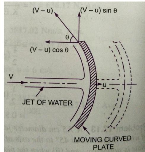
This velocity can be resolved into two components, one in the direction of jet and the other perpendicular to the direction of jet.
