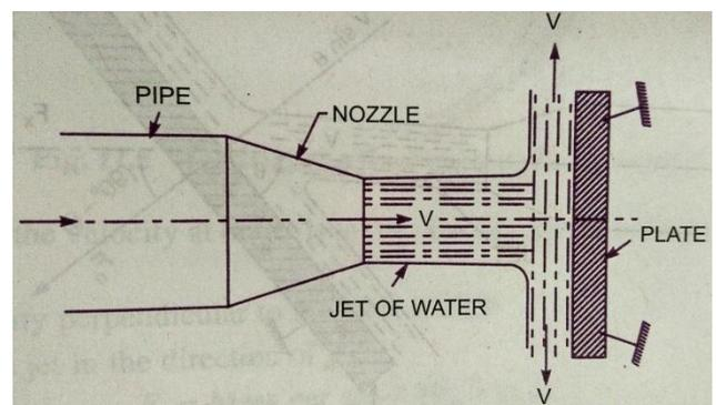
Hence the component of the velocity of the jet, in the direction of jet, after striking will be zero.
