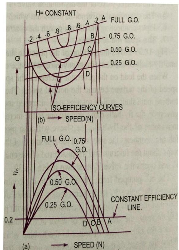
are called Iso-efficiency curves. These curves are helpful for determining the zone of constant efficiency and for predicating the performance of the turbine at various efficiencies.
