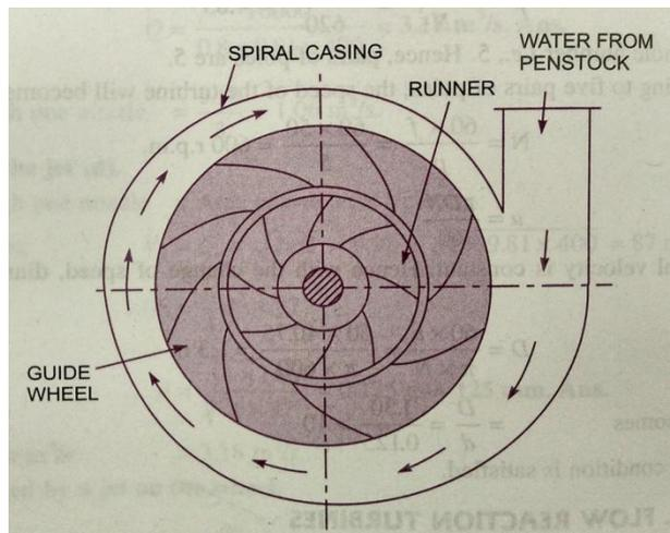
The casing completely surrounds the runner of the turbine. The water enters the runner at constant velocity throughout the circumference of the runner.
