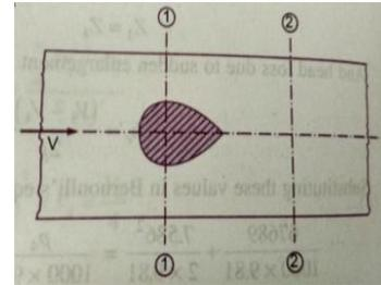
As the liquid flows and passes through section 1-1, a vena-contracta is formed beyond section 1-1- after which the stream of liquid widens again and velocity of flow at section on 2-2 become uniform and equal to velocity,  $v$  in the pipe. This situation is similar to the flow of liquid through sudden enlargement.
