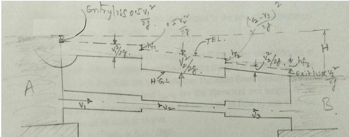
If a pipe line connecting two reservoirs is made up of several pipes of different diameters  $d_1$ ,  $d_2$ ,  $d_3$ , etc. and lengths  $L_1$ ,  $L_2$ ,  $L_3$  etc. all connected in series ( i.e. end to end ), then the difference in the liquid surface levels is equal to the sum of the head losses in all the sections. Further the discharge through each pipe will be same.
