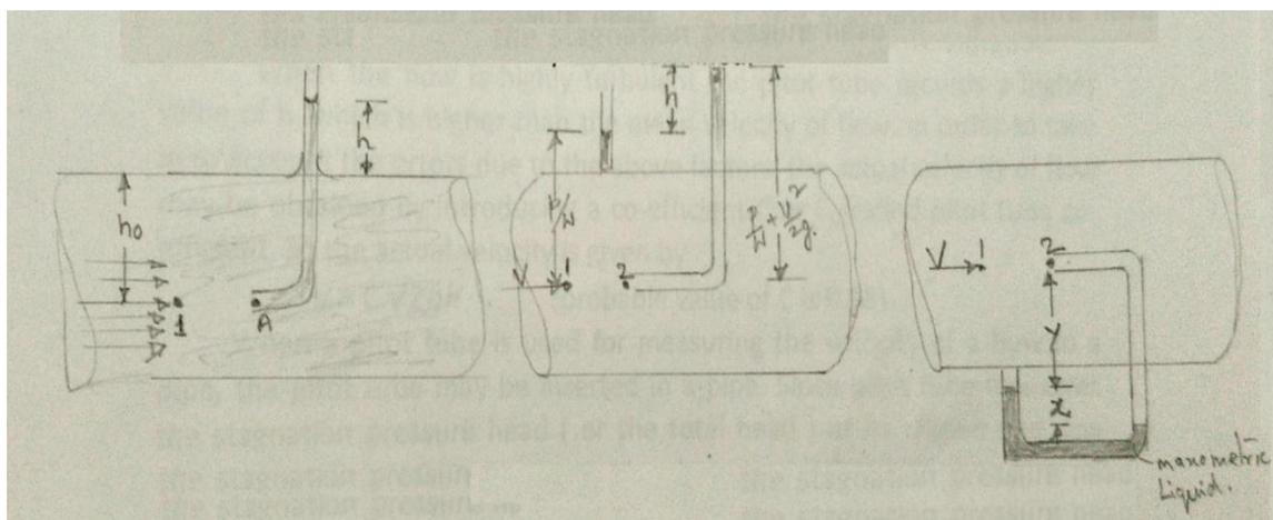
Simplest form of a pitot tube consists of a glass tube, large enough for capillary effects to be negligible and bent at right angles. A single tube of this type is used for measuring the velocity of flow in an open channel. The tube is dipped vertically in the flowing stream of fluid with its open end A directed to face the flow and other open end projecting above the fluid surface in the stream. The fluid enters the tube and the level of the
