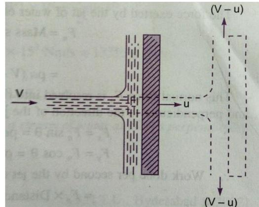
Hence relative velocity of the jet with respect to plate =  $V - u$
