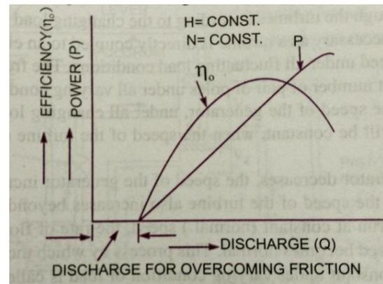
overcome initial friction. Hence the power and efficiency curves will be slightly away from the origin on the x-axis, as to overcome initial friction certain amount of discharge will be required.
