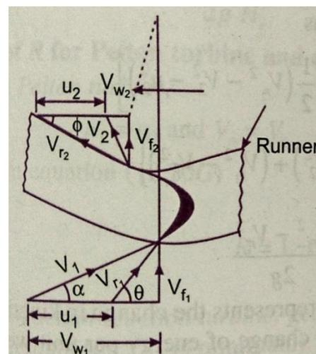
If the discharge is radial at outlet, then  $V_{w_2} = 0$
