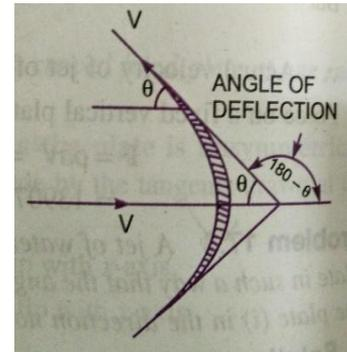
4. A jet of water of dia. 75mm moving with a velocity of 30m/sec strikes a curved fixed plate tangentially at one end at an angle of  $30^\circ$  to the horizontal. The jet leaves the plate at an angle of  $20^\circ$  to the horizontal. Find the force exerted by the jet on the plate in the horizontal and vertical direction.
