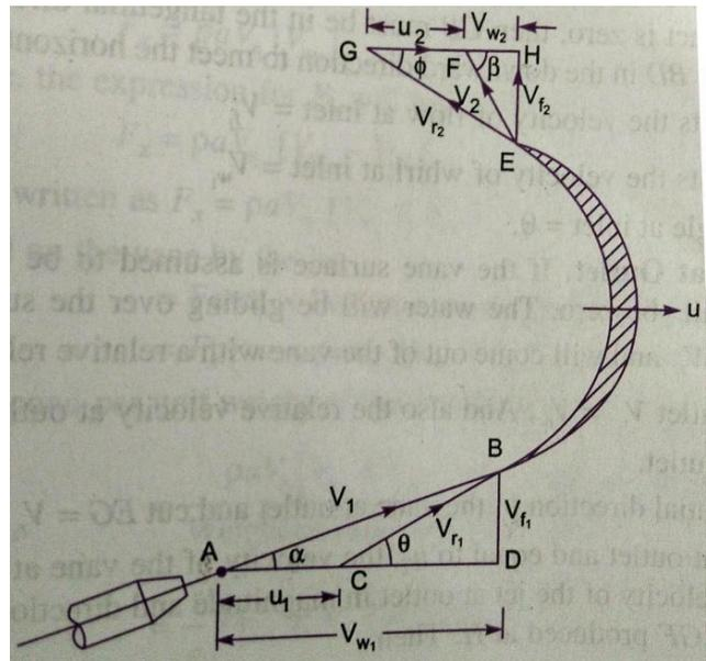
Let  $V_1$  = Velocity of jet at inlet.
