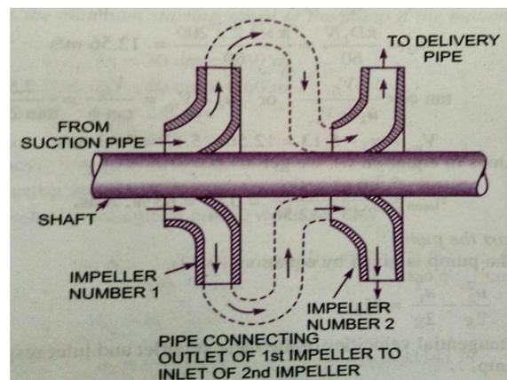
**Multi-Stage Centrifugal Pumps for High Heads:** For developing a high head, a number of impellers are mounted in series on the same shaft.
