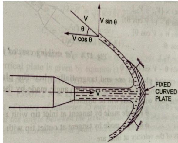
Component of velocity in the direction of jet =  $-V \cos \theta$
