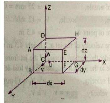
$$\frac{\partial u}{\partial x} + \frac{\partial v}{\partial y} + \frac{\partial w}{\partial z} = 0 \quad \text{_____ (8)}$$
