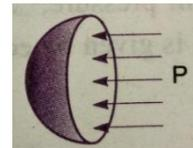
**Surface Tension on a Hollow Bubble:** A hollow bubble like soap in air has two surfaces in contact with air, one inside and other outside. Thus, two surfaces are subjected to surface tension.
