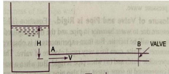
velocity, V in the pipe. If now the valve is suddenly closed, the momentum of the flowing water will be destroyed and consequently a wave of high pressure will be set up. This wave of high pressure will be transmitted along the pipe with a velocity equal to the velocity of sound wave and may create noise called knocking. Also this wave of high pressure has the effect of hammering action on the walls of the pipe and hence it is known as water hammer.
