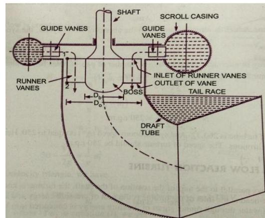
Between the guide vanes and the runner the water in the Kaplan turbine turns through a right angle into the axial direction and then passes through the runner. The runner of the Kaplan turbine has four or six or eight in some cases blades and it closely resembles a ship's propeller. The blades (vanes) attached to a hub or bosses are so shaped that water flows axially through the runner.
