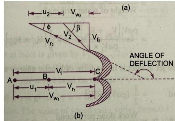
The Velocity Triangle at inlet will be a straight line where
